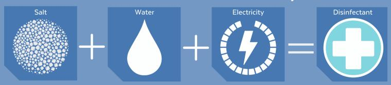
The electrolytic cell of an on-site generator uses common salt combined with water and electricity to generate high performance disinfection chemistries, eliminating the need to transport and store hazardous chemicals.
