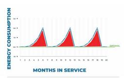
The blue line represents energy use in a conventional system that requires regular deanings. The green line shows energy use in the CES system, maintaining efficient energy use over time without cleanings. The red area between the lines is the savings to be had using the CES.
