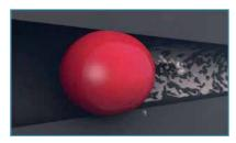
The cleaning pods flow through the tubes at normal system velocity. As water pushes them, residue, deposits and biofilm are removed, leaving clean tubes and optimal heat transfer efficiency.
