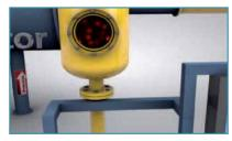
Non-abrasive cleaning pods start out in the Pod Storage Unit, connected to the condenser through the main line of the system. A window in the Pod Storage Units allows monitoring of the condition and quantity of pods inside.
